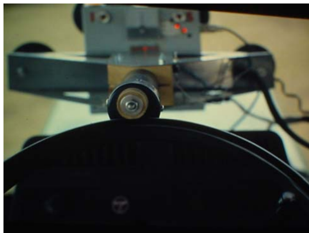
Figure 2 Auto-steering: friction drive
