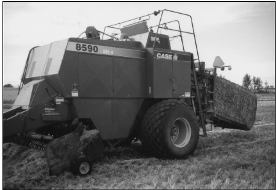
Too minimize transportation costs, large “square” bales are preferred by companies commercially harvesting crop residues.
