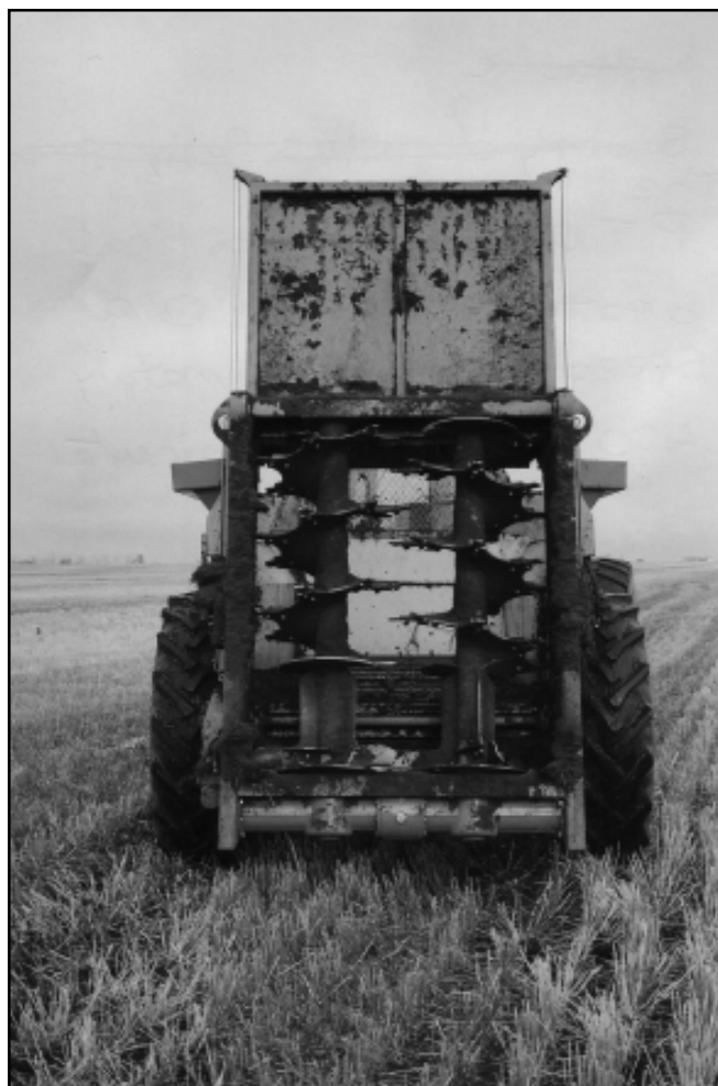
The PTO driven vertical beaters operate at a speed of approximately 400 RPM.
